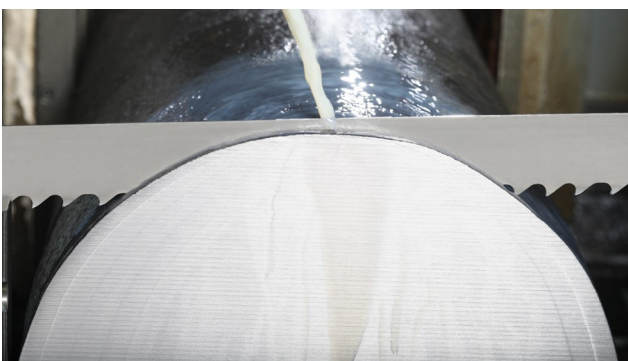
Figure 1: Flexible use: The new MARADUR® carbide-tipped band saw blade from WIKUS is suitable also for machines without a carbide package. Source: WIKUS-Sägenfabrik
